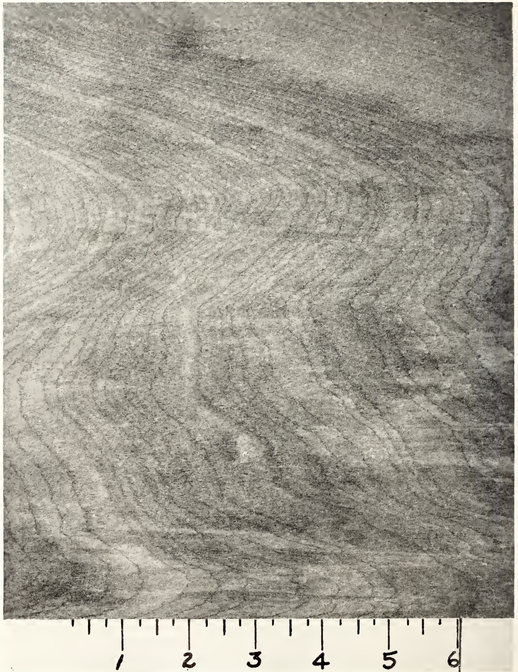
FIGURE 2-87.—Cross grain resulting from butt swell in yellow birch.
